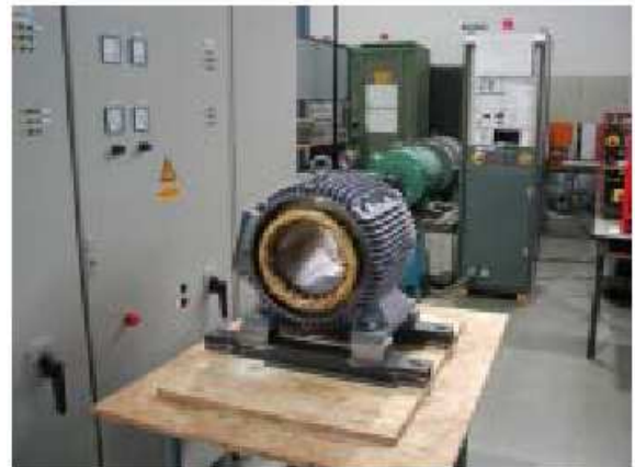
Fig.8 Three phase induction machine with cageswitching. (top) rotor with integrated power electronics (bottom) three phase stator.
