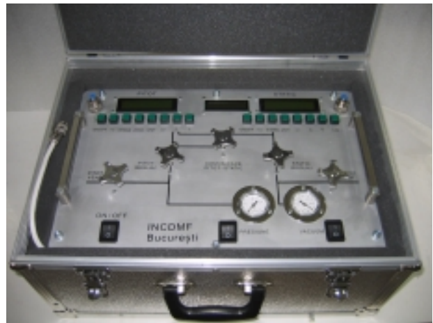
Fig. 3: Equipment for testing the tightness, the altimeters and the speedometers from aircraft's board.
