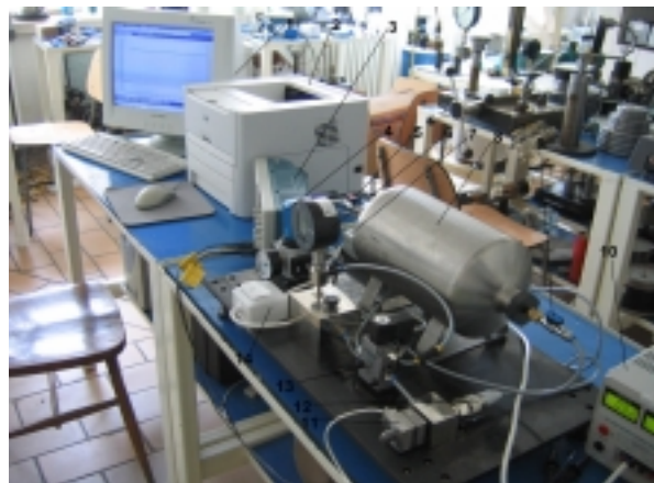
Fig. 1. Equipment For Testing & Checking The Technical Characteristics Of Pressure Transducers In A Non-Steady Regime
