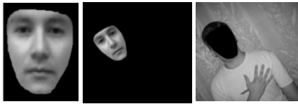
Fig. 3. The template face, the template match and the image after template matching.
