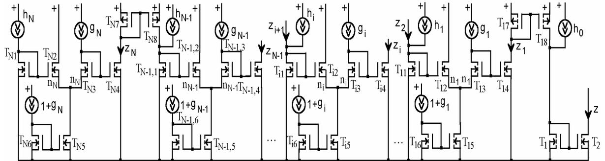
Figure 2. The CMOS translinear expandable generic network that implements the one variable polynomial approximated objective funtions.
