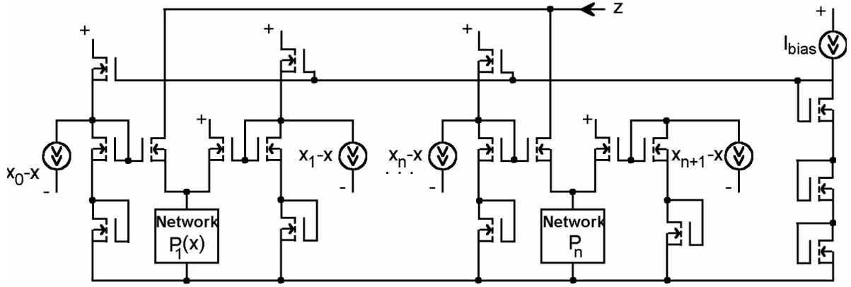
Figure 4. The network that is implementing polynomial approximated function that are not continued on the all definition interval but are continued on the subintervals that covered integer definition interval.
