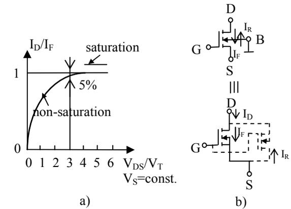
Figure 1. a) The operation regions in weak inversion of the MOS transistor; b) Non-saturated Mos transistor equivalent to two saturated transistors connected anti-parallel.
