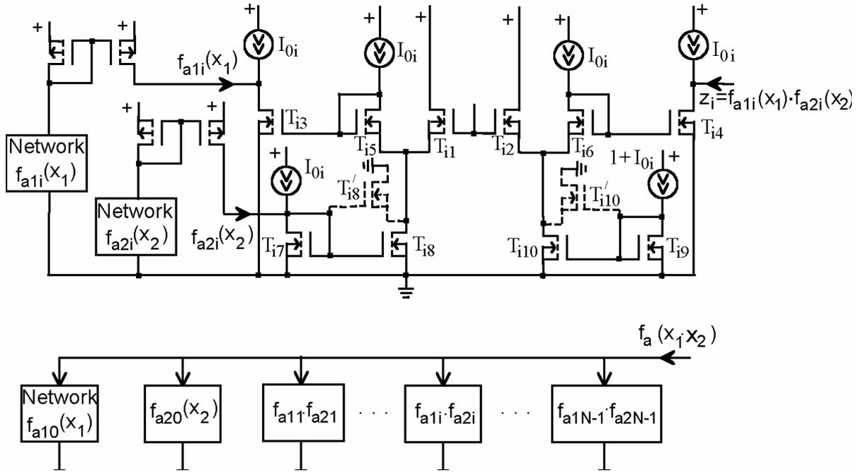
Figure 5. The network that is implementing the polynomial approximated two variable functions.
