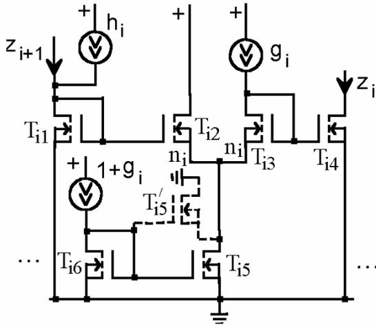
Figure 3. The  $i$  section of translinear generic network shown in figure 2.
