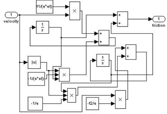
Figure 5. The Simulink Bliman-Sorine friction model
