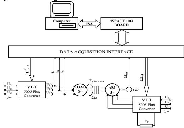
Figure 8. Hardware structure of implemented RTFS
