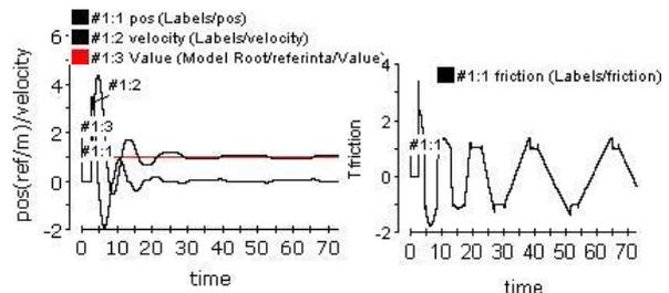
Figure 12. Position and velocity (left) and friction (right) for an emulated stick-slip motion on PID tracking control
