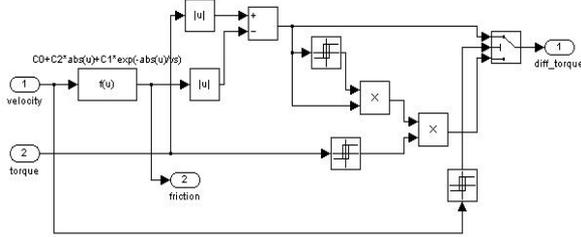
Figure 4. The Simulink Tustin friction model
