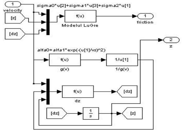
Figure 6. The Simulink LuGre friction model
