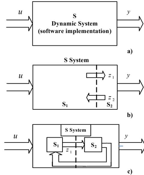
Fig. 1. BPS as a dynamic system: a) basic scheme; b) structure of system; c) SIL.
