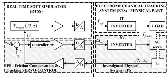
Figure 7. Simplified block diagram of the implemented RTFS
