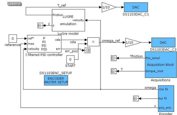
Figure 9. Main Simulink<sup>®</sup> model for friction RTSS
