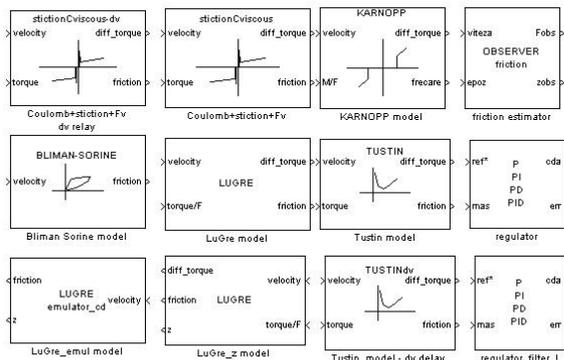
Figure 10. The Simulink® library of friction models
