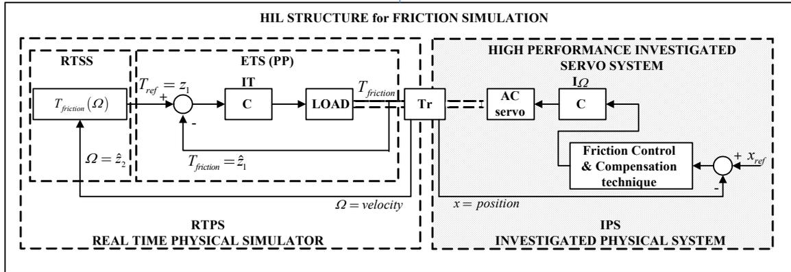
Figure 3. HIL system architecture for friction simulator
