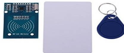
Fig. 13. MFRC522 reader / writer with MIFARE classic passive card and transponder (tag).
