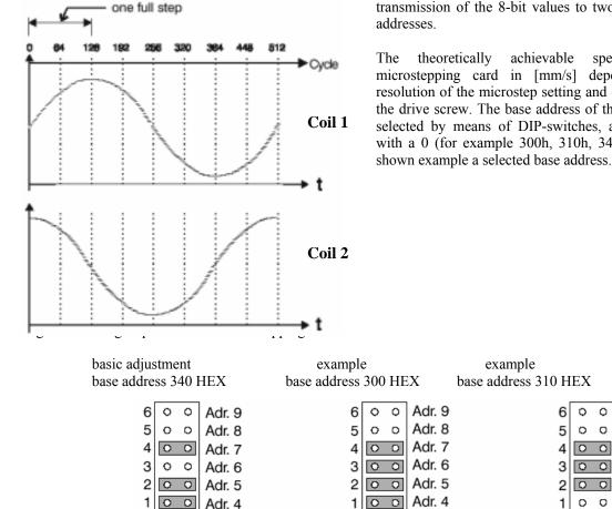
The basic principle is to produce, according to an 8bit range of 0-255, two currents 90 out-of-phase with each other, for the two phases of the motor. This is as though each motor is controlled by a two-channel current amplifier, where each current value is represented by an 8-bit value. The motor is supplied with the correct values of phase current by the transmission of the 8-bit values to two defined port
