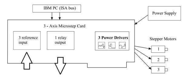
Fig.1. The block scheme of microstepping card.
