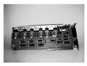
Fig.6. The general view of microstepping control card.
