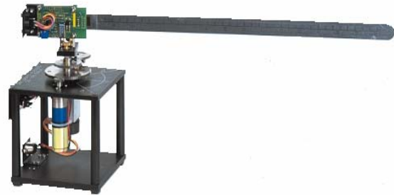
Fig. 3. Quanser Flexible Link system
