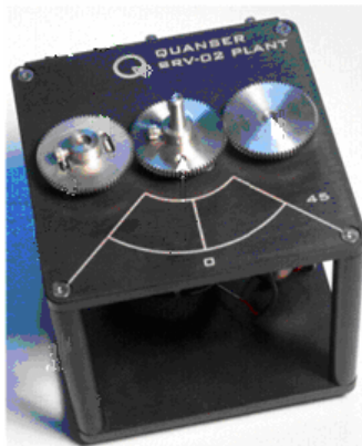
Fig. 1. SRV02 plant – DC motor and gear box
