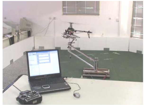
Fig. 5. The experimental test bed for autonomous helicopter flight developed in the Intelligent Systems and Robotics Laboratory of the Technical University of Crete.
