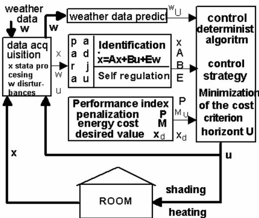
Fig. 2. The block structural schema used for controlling the air-conditioning variables in ventilated rooms.
