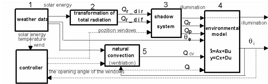
Fig. 8. The proposed simulation block structural schema, in the case of automatic control of the temperature  $\theta_i$ .
