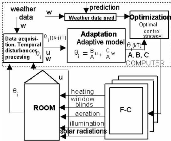
Fig. 1. The block structural schema used for controlling the air-conditioning variables with fuzzy controllers (F-C).
