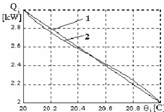
Fig. 7. The temperature control: with P controller (the curve 1); with fuzzy controller (the curve 2).
