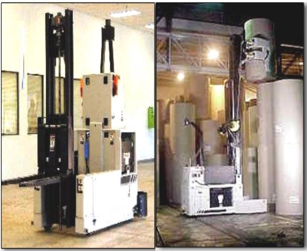
**Figure 2.** AGV forklift vehicle type.
