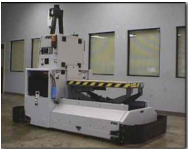
**Figure 3.** AGV unit load carrier type.
