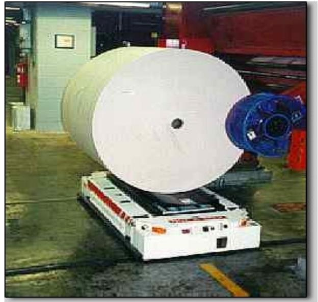
**Figure 4.** AGV unit load carrier in application.
