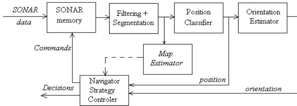
Figure 1 - The structure for the estimation of the position, using SONAR data
