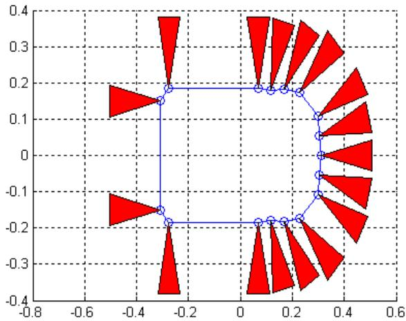
Figure 2 - Distribution of the SONAR transducers. The beam angle is about 15 degrees
