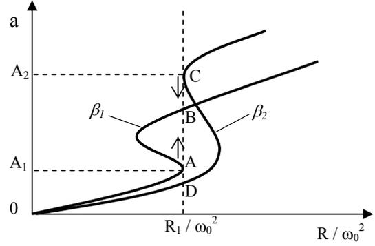
**Fig. 3** Explanatory for the resonance jump phenomenon
