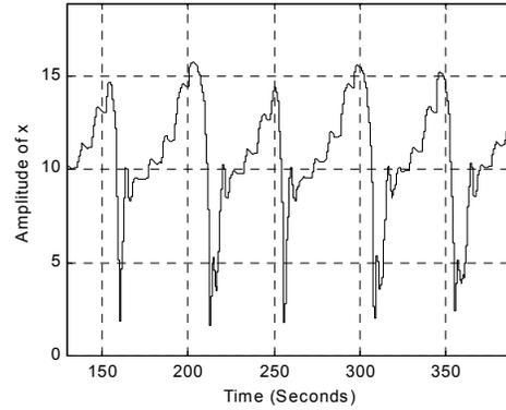
**Fig.5** Variable's  $x$  oscillations get for  $T_1=50\text{s}$ ,  $T_2=0$ ,  $\tau_1=0$ ,  $\tau_2=0$ ,  $\tau_3=0$
