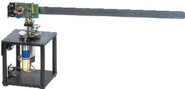
Figure 1: Quanser Flexible Link experiment
