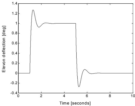
Fig. 8. The amplitude of command for elevon actuator.
