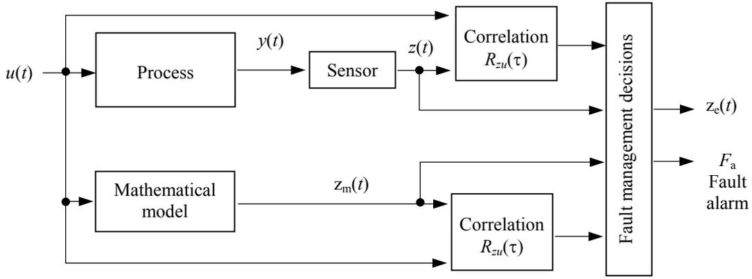
Fig. 5. The structure with one sensor and mathematical model.
