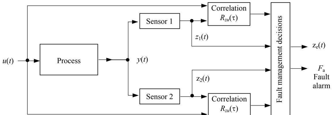
Fig 1. The structure with two sensors.
