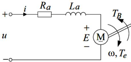
Fig. 1. DC motor equivalent circuit.
