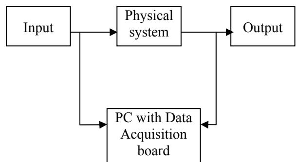
Fig. 7. System identification experimental setup
