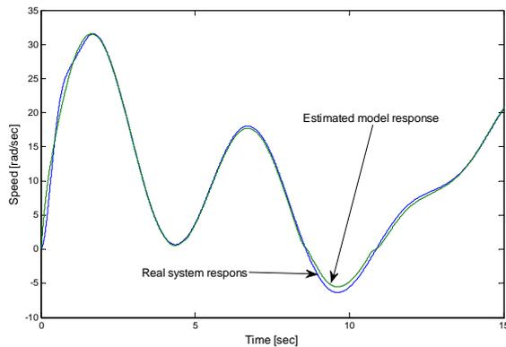
Fig. 10. Real system and estimated model responses to the same input signal
