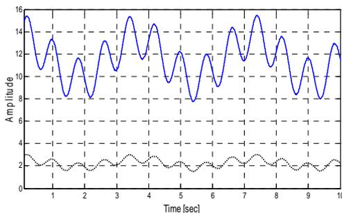
Fig. 6. System response (time evolution of state variables: speed [rad/sec] – continuous line and current [A] – dashed line)
