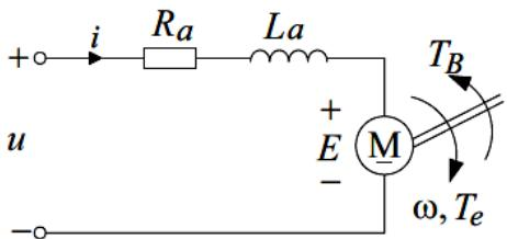
Fig. 1. DC motor equivalent circuit.
