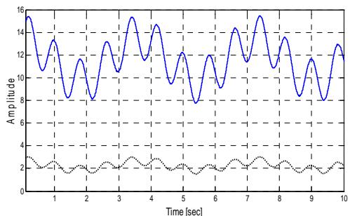
Fig. 6. System response (time evolution of state variables: speed [rad/sec] – continuous line and current [A] – dashed line)
