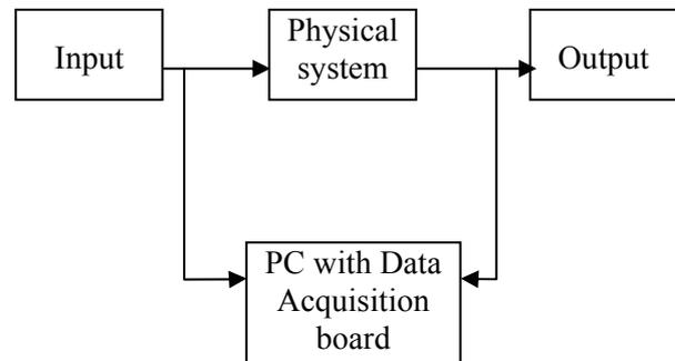
Fig. 7. System identification experimental setup
