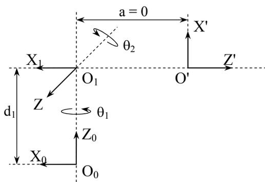
Fig. 7. First robot substructure
