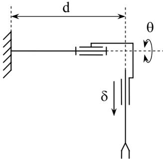
Fig. 3. Robotic kinematical structure for the Application 1
