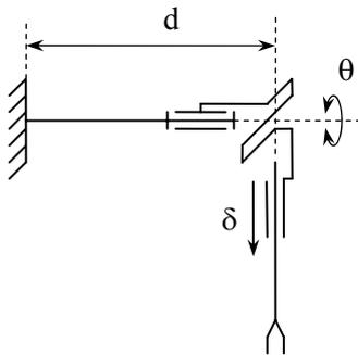
Fig. 4. Considered robotic kinematical structure
