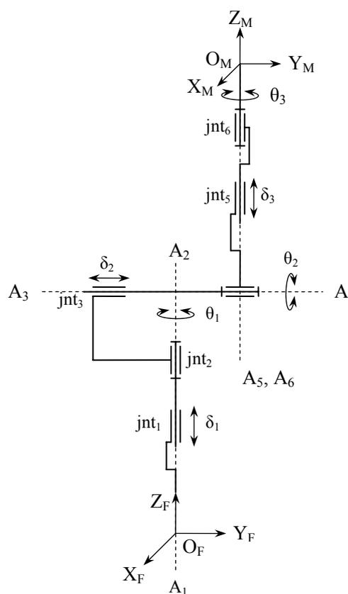
Fig. 1. Complete Kinematical Structure (CKS)
