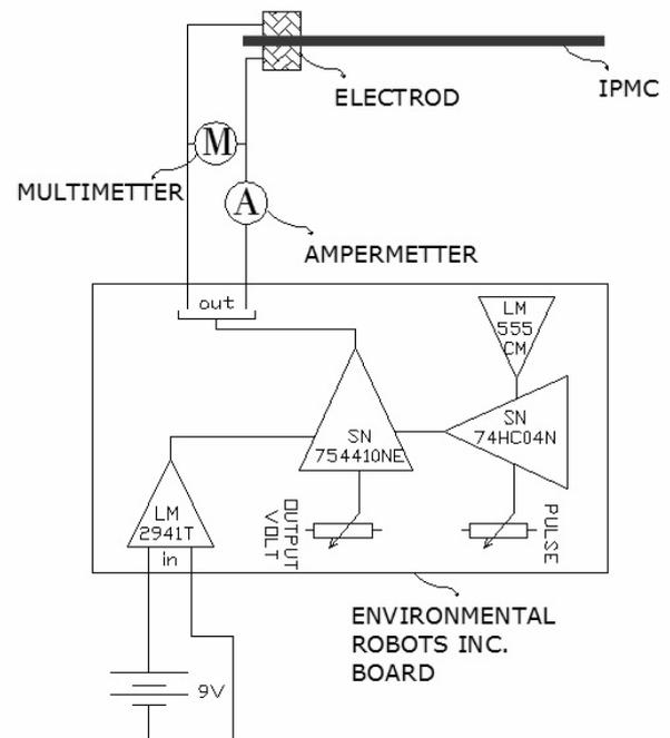
Fig. 3. Schematic representation of an experimental work stand
