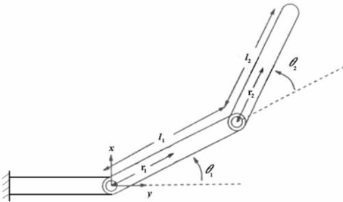
Fig. 7. Two link finger architecture
