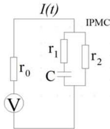
Fig. 1. RC model for a section of IPMC band
