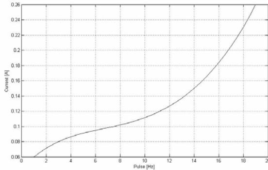
Fig. 5. Current dependency on the applied frequency, a constant voltage  $U = 1.5\text{V}$ .
