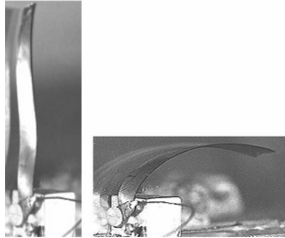
Fig. 2. IPMC in relaxed state (left) and activated state (right) (Yoseph, 2004)
