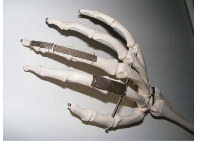
Fig. 8. Experimental structure for two link finger architecture
