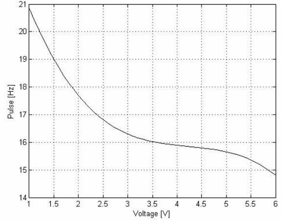
Fig. 6. Frequency variation according to voltage applied to the terminal.
