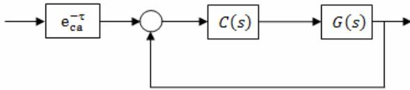
Fig. 11. The equivalent control loop
