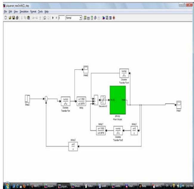
Fig. 15. The second simulation of the new Smith predictor structure
