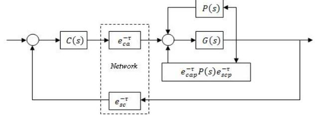
Fig.9. The control loop using the P(s) Smith predictor
