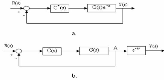
Fig. 7. The Smith controller and its equivalent conventional controller
