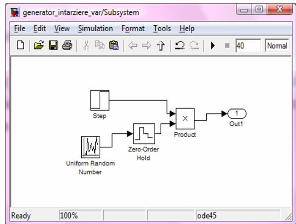
Fig.24. System for generating a uniform distributed random signal
