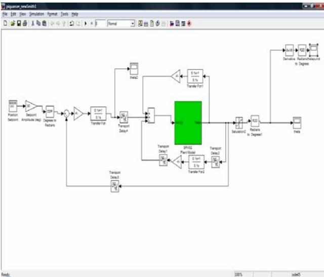
Fig. 17. Remote position control for the Quanser SRV-02 plant using the new Smith predictor configuration
