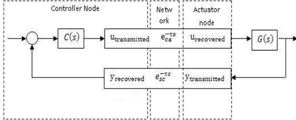
Fig. 8. The control loop with network communication delays
