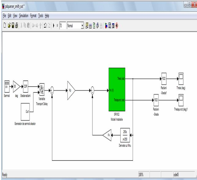
Fig. 22. Control loop using a variable delay
