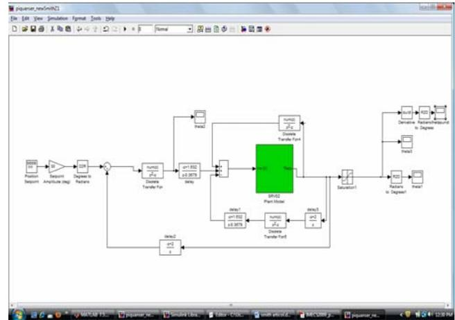
Fig. 19. Control loop with a Smith predictor and a PID discrete model controller is used
