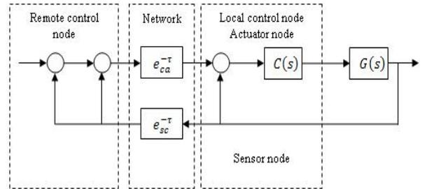
Fig. 10. The control loop using the improved P(s) Smith predictor
