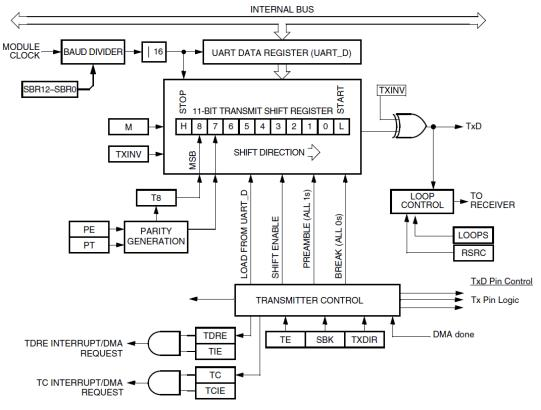
Fig. 6: FRDM-KL25Z UART transmitter block diagram (nxp.com)
