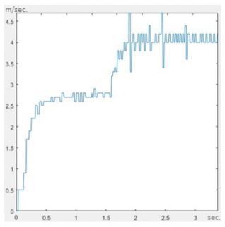
Fig. 9: DC motor response to Heaviside step
