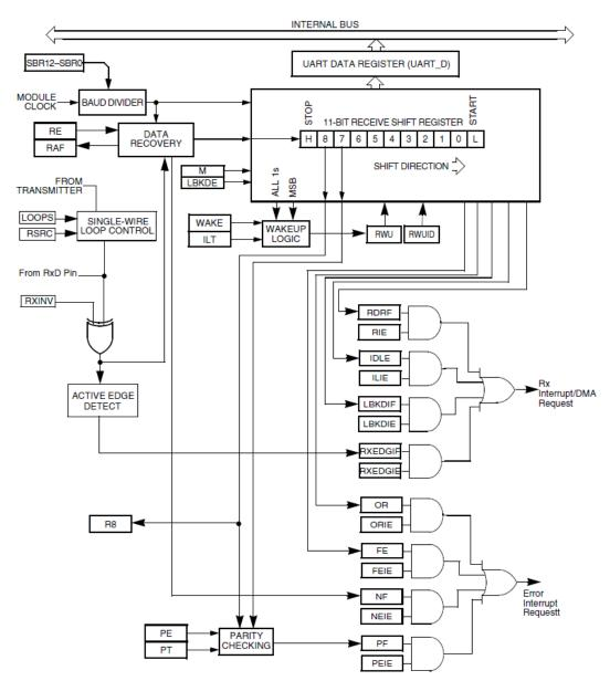
Fig. 7: FRDM-KL25Z UART receiver block diagram (nxp.com)
