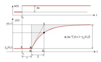
Fig. 10: Experimental determination of first order transfer function parameters
