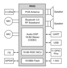
Fig. 4: RN52 Block Diagram (microchip.com)
