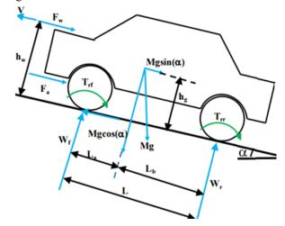
Fig. 3: Forces in the vehicle motion (nptel.ac.in)
