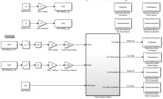
Fig. 7: Trailer system testing – Simulink block diagram
