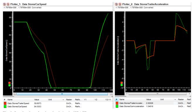
Fig. 9: Speed and acceleration simulation in dSPACE
