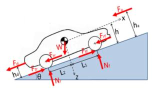
Fig. 4: Forces for longitudinal motion (ni.com)
