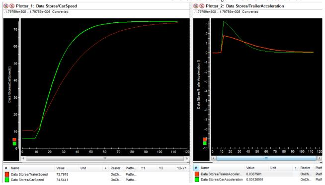
Fig. 8: Speed and acceleration simulation in dSPACE
